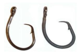
A standard circle hook (left) compared to a shark repellent hook (right). The shark repellent hook is magnetic and is covered with a special metal that produces a voltage in seawater. Credit: Eric Stroud, Shark Defense
