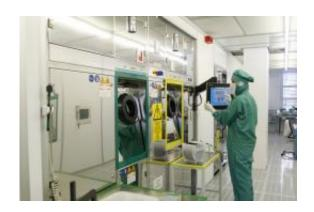
MSTs, tiny sensors integrated into semiconductor chips, are produced in the MST laboratory and clean room. A researcher operates the production machine. Credit: Fraunhofer IMS
