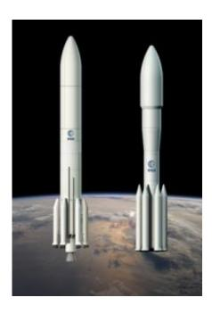
NGL concepts under study - Left: main stage powered by a cryogenic liquid oxygen and hydrogen engine (staged combustion cycle), with a cryogenic reignitable engine for the upper stage. Right: first two stages powered by solid propellants, with a cryogenic reignitable engine for the upper stage. Credits: ESA - D. Ducros
