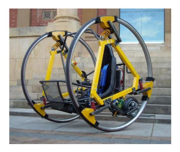
(PhysOrg.com) -- In a bit of technical wizardry, students from the University of Adelaide, Australia, have devised and built an electric diwheel, that with modification, could possibly solve inner city
