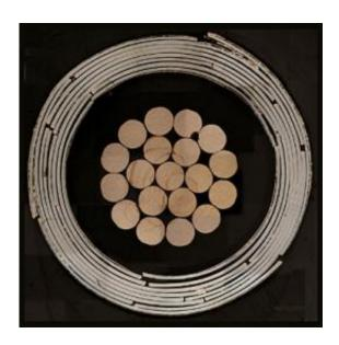
Cross-section of a high-temperature superconducting cable design invented at NIST. In the center are copper wires bundled with nylon and plastic insulation. The outer rings are a series of superconducting tapes wrapped in spirals around the copper. The cable is 7.5 millimeters in outer diameter. Credit: van der Laan/NIST
