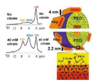
This diagram shows the effect of citrate concentration on the size of hydroxyapatite crystals fabricated with self-assembling block copolymer templates. Just as it does with actual bone structure, as the concentration of citrate increases, the thickness of the nanocrystals decreases and the thinner nanocrystals appear to make the bone more resistant to stress cracking. Credit: U.S. Dept. of Energy's Ames Laboratory
