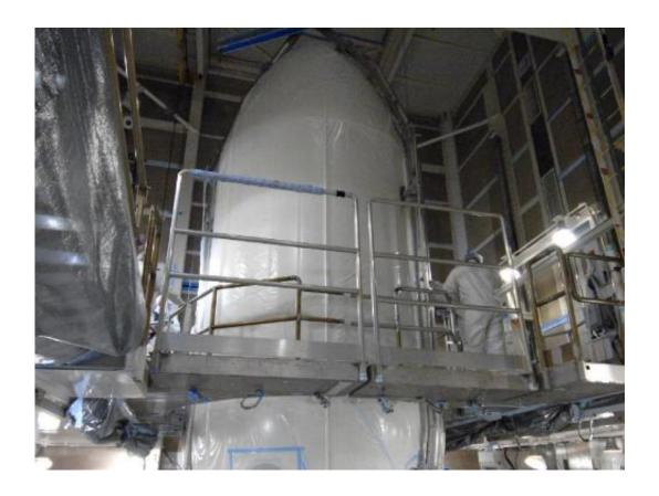
Inside the mobile service tower at Space Launch Complex-2 at Vandenberg Air Force Base in California, NASA's Aquarius spacecraft is secure inside the United Launch Alliance's Delta II payload fairing. Credit: NASA/VAFB
