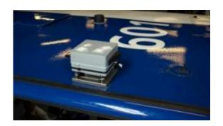
Rather than installing stations on fixed towers, why not use mobile sensors spread out over the whole city to get better air quality measurements? OpenSense, a project run by four laboratories at EPFL and one at ETH Zurich, is studying the possibility of installing sensors on the roofs of buses and trams, thus taking advantage of already existing public transport and mobile phone networks. Testing is currently underway in Lausanne.
