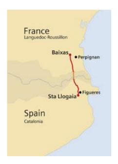
Siemens Energy is currently erecting the power converter stations for a high-voltage direct-current (HVDC) transmission link between Baixas, to the west of Perpignan in France, and Santa Llogaia, south-west of Figueras in Spain. The installation can transmit a rated power of 2000 megawatts (MW) - enough to transport large amounts of electric power with a minimum of transmission losses. The stations use the new HVDC technology HVDC Plus with a transmission voltage of ±320 kilovolts (kV)
