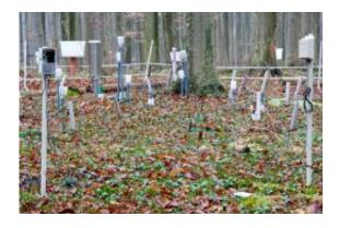
A wireless sensor network records data such as soil and leaf humidity, as well as air temperature. Credit: Fraunhofer IMS
