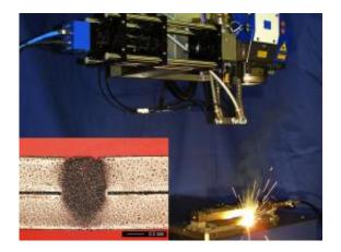
In the new surface welding process the laser produces a perfect seam. Bottom left: Weld seam profile - the penetration depth is controlled without damaging the bottom surface. (© Fraunhofer IPM)
