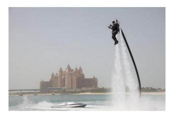
The Jetlev R200 can reach heights of 28 feet and speeds of 22 mph. Image credit: Jetlev Technologies, Inc.
