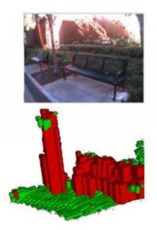
Simultaneous Localization and Mapping (SLAM) software analyzes data from stereo camera views (above) to create 3-D renderings of the scene (below), and then map a path through it. Credit: USC Viterbi School of Engineering
