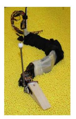
Using this robot, researchers at Georgia Tech were able to show that when its wedge-shaped head was set flat on the horizontal plane, negative lift force was generated and the robot moved downward into the medium. As the tip of the head was raised from zero to 7 degrees relative to the horizontal, the lift force increased until it became zero. At inclines above 7 degrees, the robot rose out of the medium. Credit: Georgia Tech/Daniel Goldman
