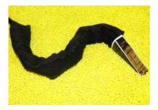
Georgia Tech School of Physics assistant professor Daniel Goldman and his team were able to show that by tilting this undulating robot's head up and down slightly, they could control the robot's vertical motion as it traveled forward within a granular medium. The robot is built with seven connected segments, powered by servo motors, packed in a latex sock and wrapped in a spandex swimsuit. Credit: Georgia Tech/Daniel Goldman
