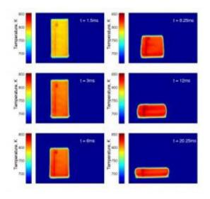
A piece of metallic glass being heated and squished in milliseconds, as seen in these infrared snapshots. Credit: Joseph P. Schramm
