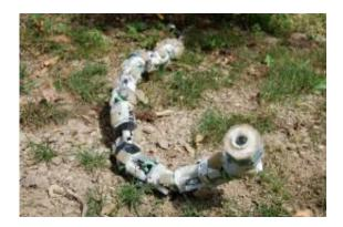
Howie Choset has developed a snake robot that moves without the aid of a fixed base. It can coordinate internal degrees movement to do a variety of locomotion capabilities. Credit: Howie Choset, Carnegie Mellon University
