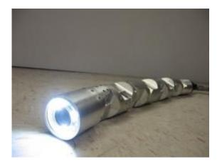
Choset added sensors, a camera and a light so that the robotic snake can function for a number of different conditions. One of its main functions will be to serve as a tool for search and rescue. Credit: Howie Choset, Carnegie Mellon University
