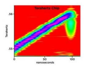
Graph shows the NIST detector's linear increase in frequency as a function of time, sweeping from 550-561 Gigahertz in frequency over 100 nanoseconds. Click on the image to see an animation of the process, slowed to 5 seconds and using an audio chirp as an analogy to the terahertz chirp. Credit: Plusquellic, NIST
