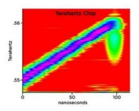
Graph shows the NIST detector's linear increase in frequency as a function of time, sweeping from 550-561 Gigahertz in frequency over 100 nanoseconds. Click on the image to see an animation of the process, slowed to 5 seconds and using an audio chirp as an analogy to the terahertz chirp. Credit: Plusquellic, NIST
