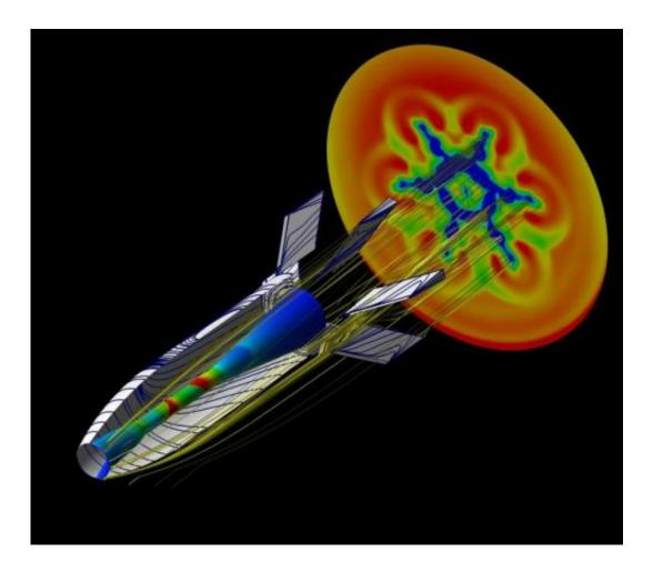
Computer-simulated flow patterns in and around the scramjet (image credit Dr Melrose Brown)
