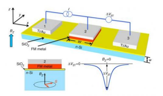
Measurement geometry. In the three-terminal device measurement geometry, a current is applied to contacts 1 and 2, and a voltage is measured across contacts 2 and 3. Electrical spin injection produces spin accumulation in the transport channel under the magnetic contact 2 and a corresponding output voltage. When a magnetic field Bz is applied, the injected spins precess and dephase, and the spin accumulation decreases to zero. U.S. Naval Research Laboratory
