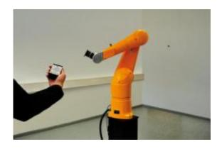
The robotic arm can be controlled with an input device. When the hand holding the device is moved, the robot emulates the movement. Credit: Fraunhofer IPA
