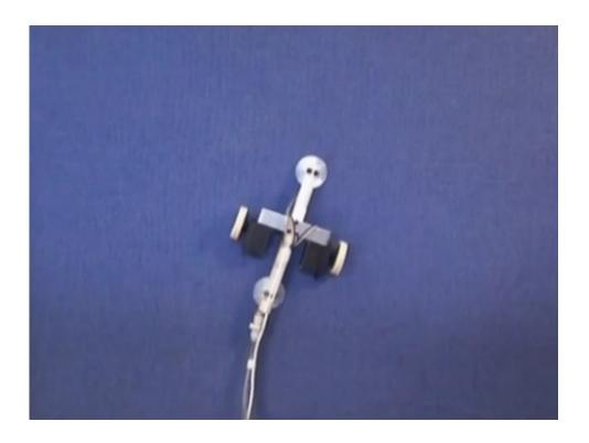
In this clip from the video below, the robot crawls up a wall using a non-contact vacuum grip, due to Bernoulli's principle. Image credit: University of Canterbury.
