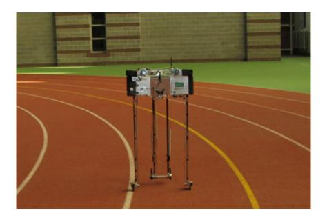
The robot Ranger, which set an untethered walking record in Barton Hall.
