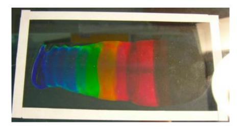
This multicolored image shows the range of colors that can be made by mixing the two block copolymers in varying proportions. Credit: University of Sheffield
