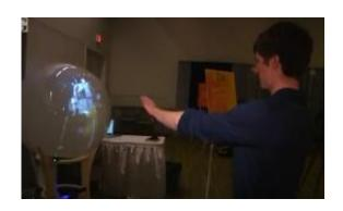
(PhysOrg.com) -- It seems like lately everyone is playing around with the Microsoft Kinect to make something different than the in the box configuration. This time the modifications are coming students at Queens University. They have combined a pair of the Kinect sensors with a hacked 3D HD projector and a hemispherical mirror mounted inside of an acrylic sphere to make a pseudo holographic display.
