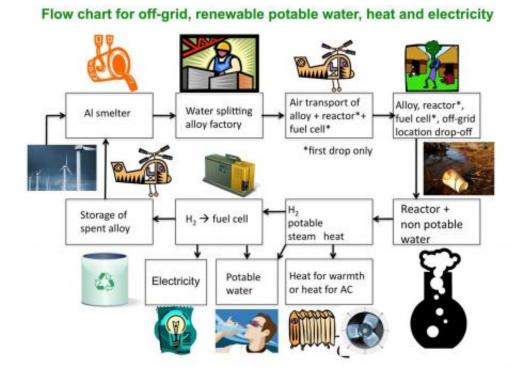
A cartoon illustrates the potential uses of a new theoretical type of mobile technology that would use an aluminum alloy to convert non-potable water into drinking water while also extracting hydrogen to generate electricity. Such a lightweight, portable system might be used to provide power and drinking water to villages and also for military operations. Credit: Jerry Woodall, Purdue University
