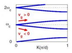
The band structure of a photonic crystal supports pulse propagation in opposite directions, as indicated by the red arrows. Scientists have described a scheme that uses this band structure to time-reverse pulses with 100% efficiency. Image credit: Sivan, et al. ©2011 American Physical Society
