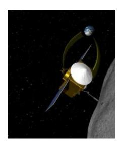
OSIRIS-REx will rendezvous with asteroid 1999 RQ36, extend a sample collecting device and return at least 60 grams (a little over 2 ounces) of pristine material to Earth for analysis. Credit: NASA/GSFC/The University of Arizona
