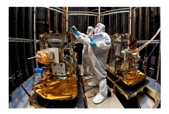
Technicians prepare to hoist one of the two Grail spacecraft upon completion of a thermal vacuum test at the Lockheed Martin Space Systems facility in Denver. Credit: NASA/JPL-Caltech/LMSS
