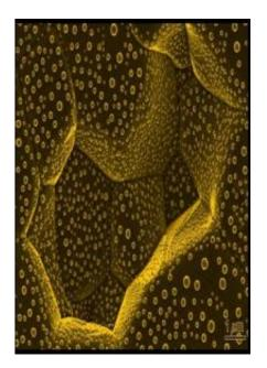
Gold crystals equilibrated on a polycrystalline sapphire(aluminum oxide) surface.
