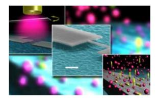
Left: an illustration of the nozzle spraying diffuse xenon gas onto the device. Middle: a close-up image of the bridgelike resonator. Right: an illustration of the atoms sticking, unsticking, and sliding off the device surface. Credit: Philip Feng. Modified image reprinted with permsision from Nano Lett., 2011, 11 (4), pp. 1753-1759. Copyright 2011 American Chemical Society.
