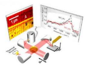
Infrared nanospectroscopy with a thermal source. The tip is illuminated with the broadband infrared radiation from of a thermal source and the backscattered light is analyzed with a Fourier spectrometer, yielding local infrared spectra with a spatial resolution better than 100 nm. The displayed graph shows infrared spectra of differently processed oxides in an industrial semiconductor device. Credit: Copyright F. Huth, CIC nanoGUNE.
