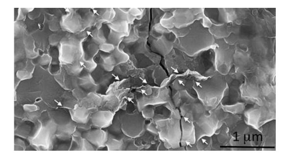
Wrapping of graphene platelets around silicon nitride grain boundaries. The graphene platelets are able to deflect propagating cracks thereby toughening the ceramic by over 200 percent. Credit: Nikhil Koratkar, Rensselaer Polytechnic Institute and Erica Corral, University of Arizona
