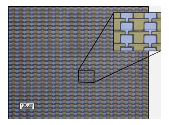
Optical micrograph of an array of graphene transistors prepared on silicon carbide (SiC). There are 40,000 devices per square centimeter. Credit: M. Sprinkle, M. Ruan, Y. Hu, J. Hankinson, M. Rubio-Roy, B. Zhang, X. Wu, C. Berger & W. A. de Heer. (2010). Scalable templated growth of graphene nanoribbons on SiC. Nature Nanotechnology (5), 727-731.
