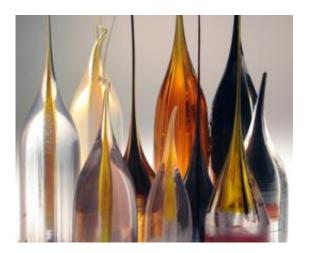
Samples of materials that have been made into fibers in the lab of MIT's Yoel Fink. The initial material is made into a 'preform,' in the lower portion, which is then heated and drawn out like taffy into a fiber from the top, preserving the arrangement of materials within the structure. Photo: Greg Hren/RLE
