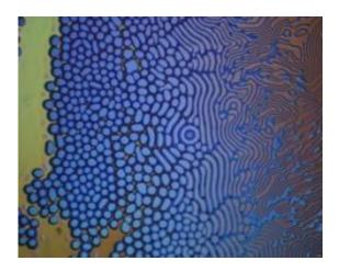
Transition between 3-D nanopillar arrays and striped structures in a polystyrene nanofilm subject to a thermal gradient of 100,000 degrees Celsius/cm. [Credit: Courtesy of E. McLeod and S. M. Troian, {LIS2T} lab/Caltech]
