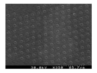
Scanning electron micrograph of solidified protrusions in a 98 nm polystyrene film guided by a remote hexagonal array of cold pins. [Credit: Courtesy of E. McLeod and S. M. Troian, {LIS2T} lab/Caltech.]
