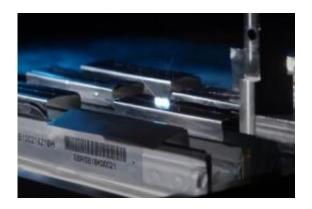
The welding of aluminum and copper battery lugs with a disk laser for the production of battery systems used in electric vehicles. Credit: Fraunhofer ILT
