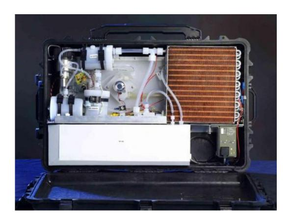
A team of scientists at NASA's Jet Propulsion Laboratory originally developed this 300-watt engineering prototype of a Direct Methanol Fuel Cell system for defense applications. Credit: NASA/JPL-Caltech
