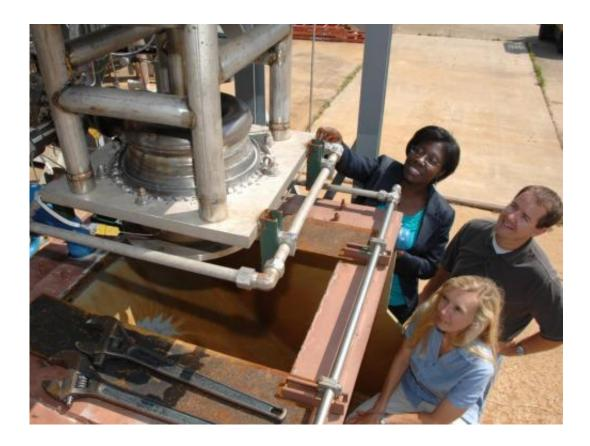
Engineers, from left, Lakiesha V. Hawkins, David C. Reynolds, and Cynthia L. Sprader inspect the J-2X fuel turbopump first stage nozzle after a successful test series in Marshall's Test Stand 116. Credit: NASA/MSFC/D. Olive
