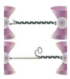
The figure shows a double-stranded DNA molecule, which is held suspended between to optical tweezers. When the tweezers pull at the molecule it will first stretch, twist and finally melt into 'bubbles'.
