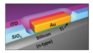
An optical antenna-diode for photodetection. Representation of a single Au resonant antenna on an n-type silicon substrate. For more information, please see Figure 1 in the manuscript. Credit: Science/AAS
