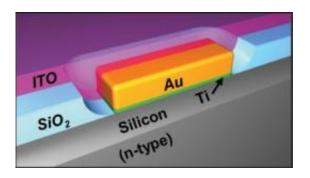
An optical antenna-diode for photodetection. Representation of a single Au resonant antenna on an n-type silicon substrate. For more information, please see Figure 1 in the manuscript. Credit: Science/AAAS
