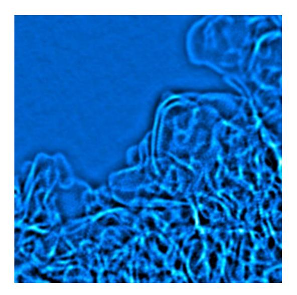
Atomic resolution electron micrograph of activated graphene. The images (this one and another one below) show that the material is composed of single sheets of crystalline carbon, which are highly curved to form a three-dimensional porous network.
