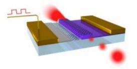
This is a schematic illustration of the graphene-based optical modulator. A layer of graphene (black fishnet) is placed on top of a silicon waveguide (blue), which is used as an optical fiber to guide light. Electrical signals are sent in from the side of the graphene to alter the amount of photons the graphene absorbs. Credit: Graphic by Ming Liu, UC Berkeley
