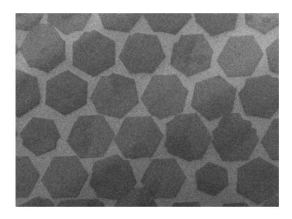
This scanning electron microscope picture shows individual crystal "grains" in an array of a material called graphene. Researchers have developed a method for creating the arrays, an advancement that opens up the possibility of a replacement for silicon in high-performance computers and electronics. (Image Care of University of Houston)
