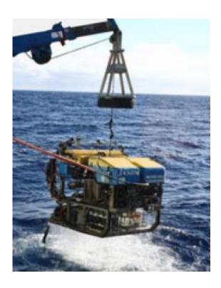
Jason II, a remotely operated vehicle, or ROV, was also used to sample pyrite nanoparticles. Credit: Mustafa Yucel
