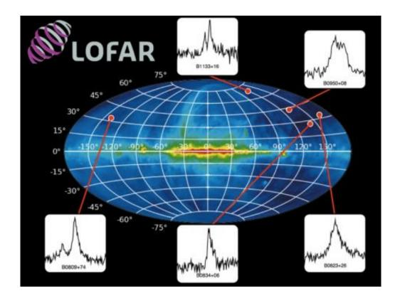
Its unique design allows Lofar to simultaneously detect radio emission from different directions. This image was obtained with Lofar by simultaneously observing five pulsars distributed across the whole sky. Credit: Tom Hassall / U.Man. / ASTRON
