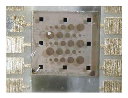
The researchers' experimental setup consisted of a sample of the lanthanum aluminate-strontium titanate composite, which looks like a slab of thick glass,
