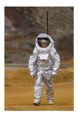
Aouda.X, a spacesuit mockup, was tested with the Long Term Medical Survey System (LTMS) in Mars-like terrain of Spain's Rio Tinto in April 2011. The suit was developed by the Austrian Space Forum to simulate the functions and feel of a spacesuit that would possibly be used by astronauts on a planet. Credits: ESA
