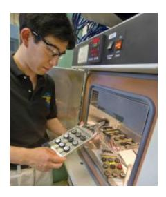
Berkeley Lab battery scientist Gao Liu inspects coin cells cycling in an environmental chamber.
