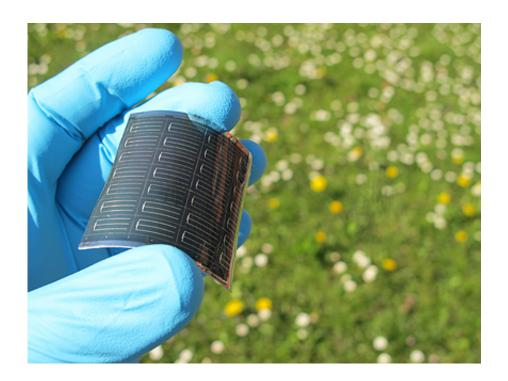
Flexible thin film CIGS solar cell on polymer substrate developed at Empa (Copyright: Empa)
