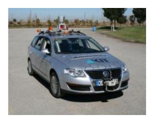
Equipped with sensors and computers, AnnieWAY autonomously finds its way in road traffic. Credit: Photo: KIT
