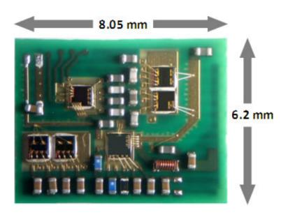
NTT DOCOMO today announced that it has developed a prototype power amplifier for six frequency bands between 1.5 GHz and 2.5 GHz in a form factor smaller than multiple single-band power amplifiers conventionally used to provide the same function.
